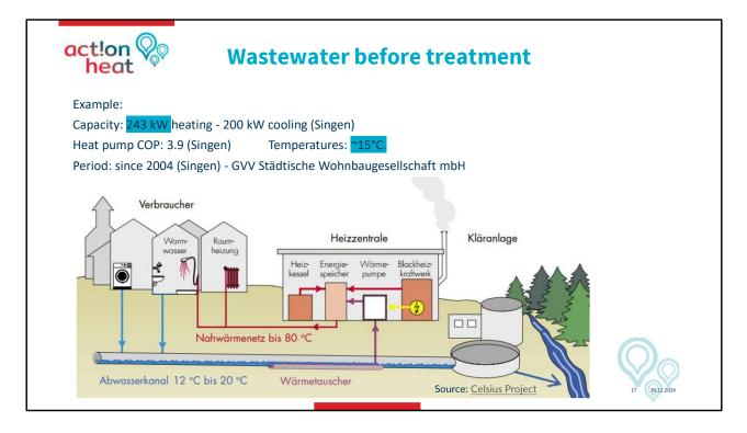
Waste water before and after treatment are low temperature
