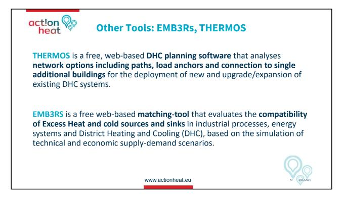
Tools for analysing the use of Excess Heat
