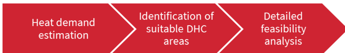
Figure 2.1 - Steps in the integrated use of Hotmaps and THERMOS for the definition of concrete DHC feasibility analyses
